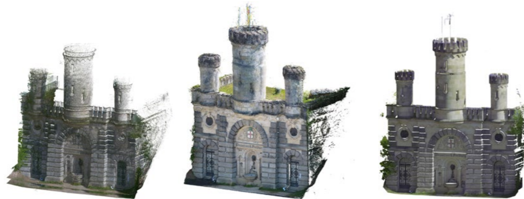
Figure 6: Individually generated 3D point clouds with (from left to right): 1. data from the handheld scanner (BLK2GO), 2. photogrammetric data captured with the Phantom 4, 3. data from the terrestrial scanner (RTC360) © Fraunhofer IPM
