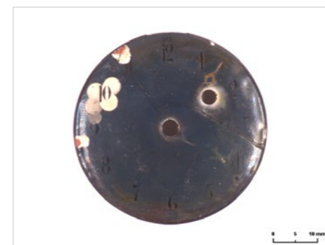
Figure 26: Fire damaged enamel dial of a pocket watch from SKD (inventory no. D IV a 450) with laser cleaned test spots © SKD
