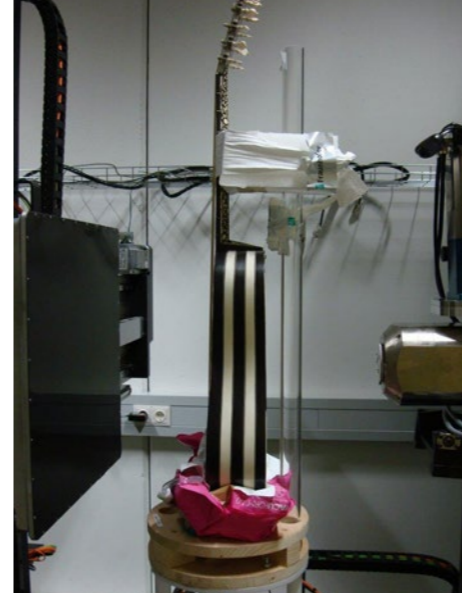
Figure 8: A guitar (Germanisches Nationalmuseum, MI58) prepared for scanning on the multifunctional mounting system. The instrument is fixed on a rotational table (center) between the X-ray source (metal tube case, right) and the X-ray imaging sensor (black square, left). While the object is rotating slowly in the X-ray beam, several hundred up to thousands of images are recorded and processed afterwards by the image reconstruction computer, which calculates the three dimensional volume image, the so-called "voxel data set". © Germanisches Nationalmuseum, Nürnberg
