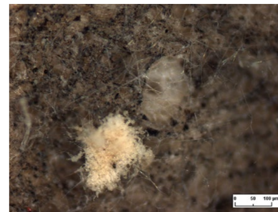
Figure 20: Light micrograph, magnification 155x, fungal hyphae and fungal spores on the paper surface © Fraunhofer FEP
