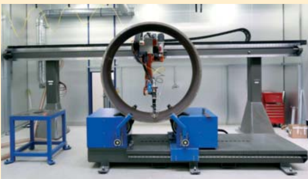
System for large area laser buildup welding of container parts with IWS wide jet processing optics
