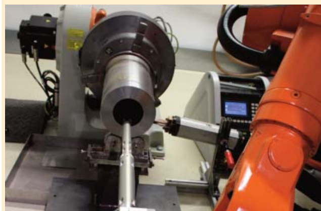
Welding setup for inductively assisted inner diameter cladding
