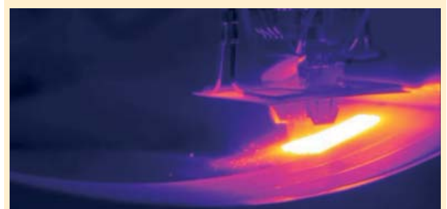
Thermal image during laser powder buildup welding with 15 kW laser power and wide jet nozzle
