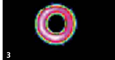
False color image of a laser beam hardening process with a ring shaped laser beam spot, recorded with the "E-MAqS" system
