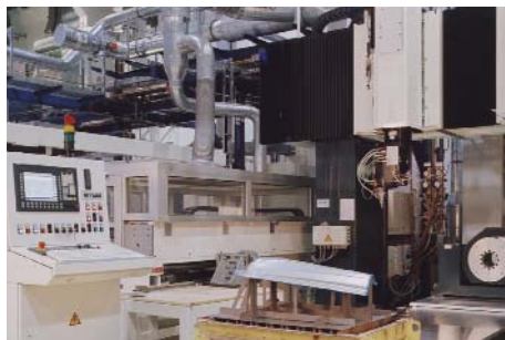
High-speed 3D laser cutting system with linear drives
