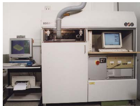
System for the rapid prototyping through direct laser liquid phase sintering
