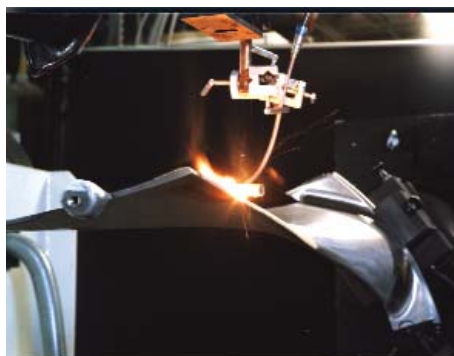
Process of the surface hardening of a turbine blade
