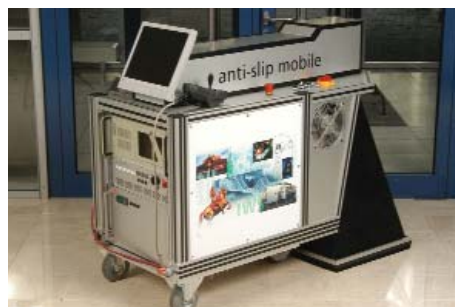
Mobile system for the anti-slip preparation of natural stone
