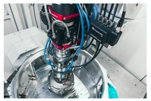
POWDERscreen is designed for laser cladding, whereby special nozzles deliver concentrated streams of metal powder precisely into the focus of a laser beam. This melts the powder onto the workpiece surface to create complex 3D structures.
