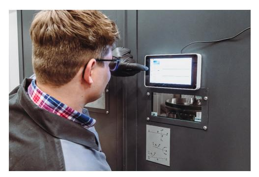
POWDERscreen can be integrated into modern industrial environments or solutions for the Industrial Internet of Things (IIoT) via its interfaces. For example, analog data output is possible via a voltage interface, via the "Message Queuing Telemetry Transport" (MQTT) protocol or data transfer via software.
