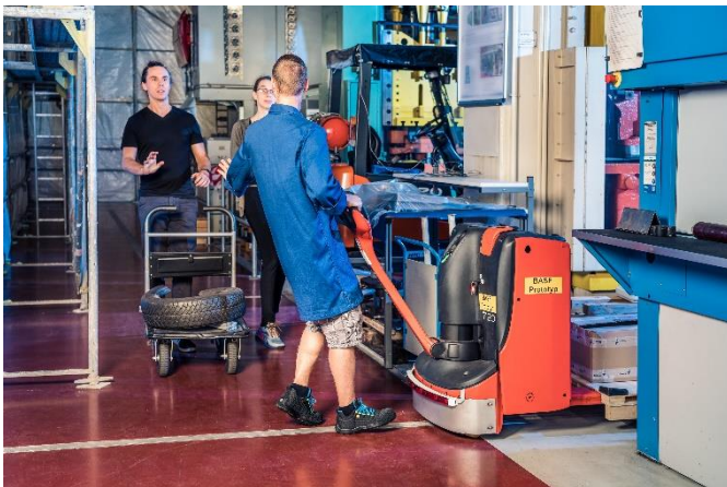
Fig. 2 A specially developed proximity sensor is used to protect the user from crushing, especially in the area around the feet. It detects when the operator moves too close to the danger zone ahead of the vehicle and stops it.
