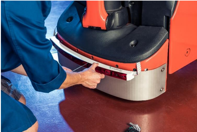
Fig. 3 Specifically designed optical sensors from the Fraunhofer Application Center AZOM aim to reduce transport accidents involving industrial trucks.
