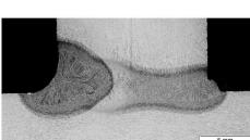
The cross-sections of a butt joint and a T-joint produced using laser MPNG show the seam quality that can be produced with significantly reduced costs and re-source consumption.
