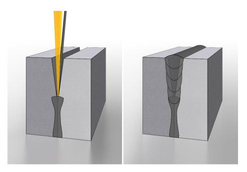
The laser beam is positioned at the joint be-tween the two sheet edges to be welded, and a filler metal is inserted in front of it at the same time. The process results in a high-quality welded seam. © Fraunhofer IWS
