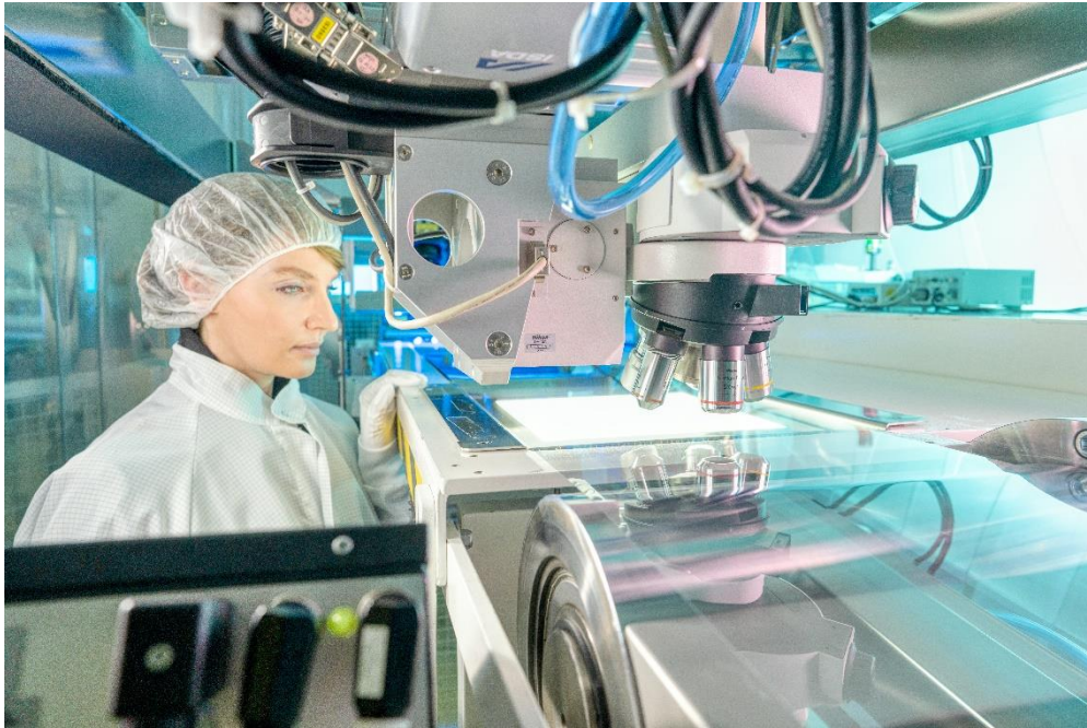
Roll-to-roll foil inspection system at Fraunhofer FEP. © ronaldbonss.com
