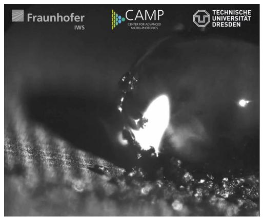
Water drops do not adhere to the self-cleaning aluminium surface. The latter has been functionalized by a team of "CAMP" scientists using direct laser interference patterning (DLIP). © Fraunhofer IWS Dresden
