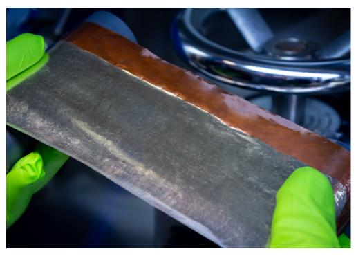
Lithium coating on copper foil created by IWS melt deposition: The process already permits producing prototype cells with lithium anode layers of 5 to 30 micrometers in thickness.
