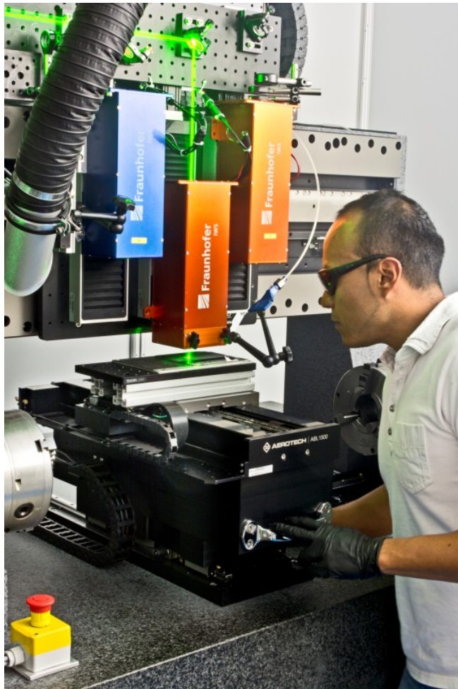
Alfredo Aguilar, Scientist with the team Surface Functionalization at Fraunhofer IWS, operates the world's largest 3D DLIP system based at TU Dresden.
