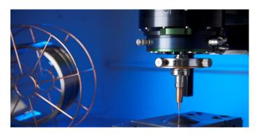
The COAXwire laser processing head can be optionally equipped with hot-wire module. © Jürgen Jeibmann
