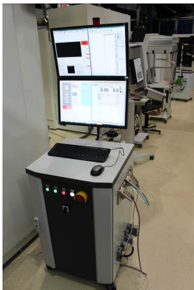
Fig. 3: remoweld ®MPNG-control tower
