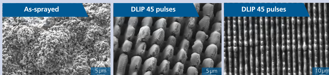
Top surface SEM-micrographs of as-sprayed and laser-treated \text{TiO}_2 coatings after DLIP treatment with different laser conditions.
